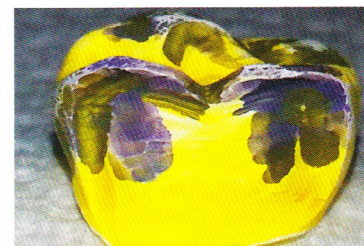
Figure 9: Milled zirconia molar Beauty and the Beast crown with colorant applied before sintering.
